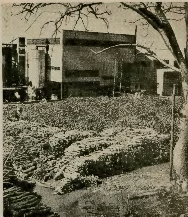
Inside NEPA mills : Heaps of peeled 'sabal' logs to be taken to the grinders.
