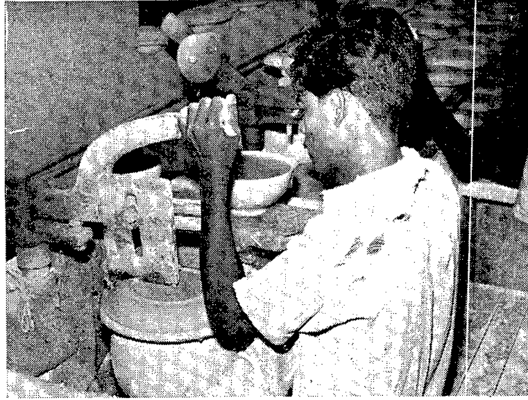
Left : Extruding pipes at the rate of four a minute, Below : A plate being cut on a jigger.
